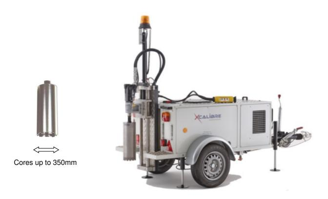
'T4' is a self contained hydraulically driven diamond drilling trailer for taking core samples in roads or airport runways with concrete or asphalt surfaces. Rugged, compact, manouverable coring trailer which out performs all manually fed or direct engine driven machines.
